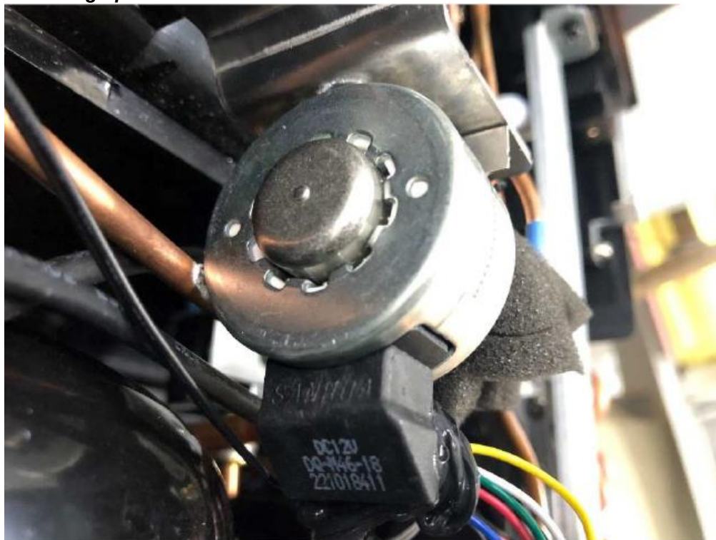
Fig.31- Solenoid valve
