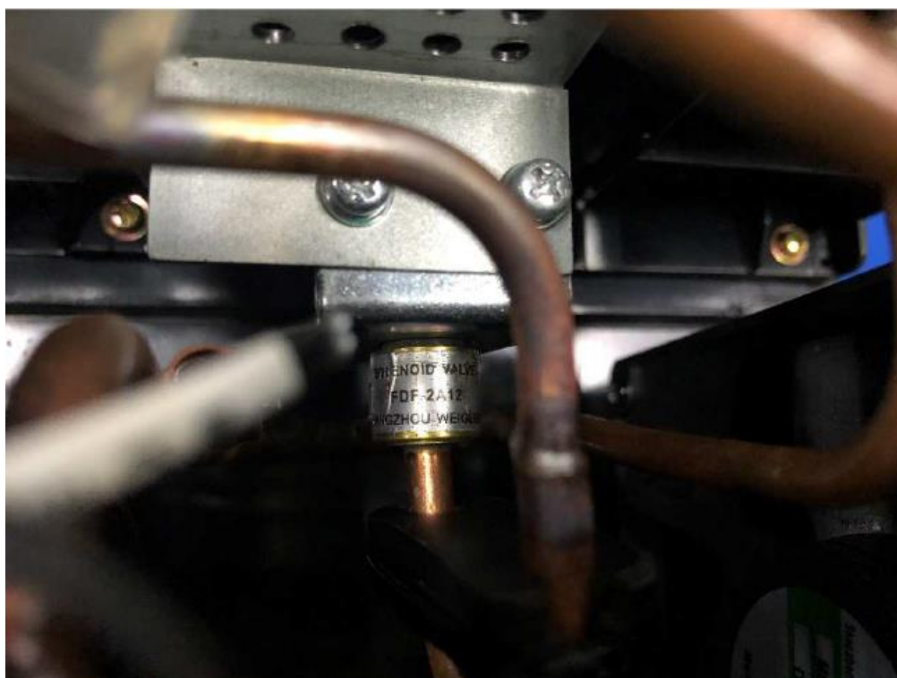
Fig.32- Ice melting solenoid valve
